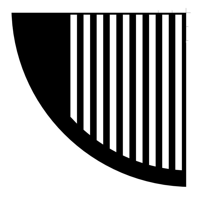
Bahtinov Focusing mask for 15" f/5 telescope - www.deepskywatch.com A4 printout, generated by "Astrojargon.net" tool
